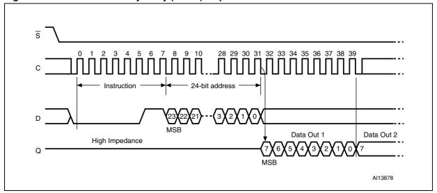
Figure 12. Read from Memory Array (READ) sequence
