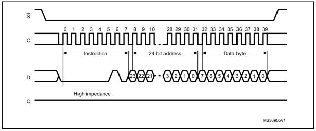
In the case of *Figure 13*, Chip Select  $(\overline{S})$  is driven high after the eighth bit of the data byte has been latched in, indicating that the instruction is being used to write a single byte. However, if Chip Select  $(\overline{S})$  continues to be driven low, as shown in *Figure 14*, the next byte of input data is shifted in, so that more than a single byte, starting from the given address towards the end of the same page, can be written in a single internal Write cycle.
