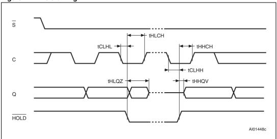
Figure 22. Serial output timing
